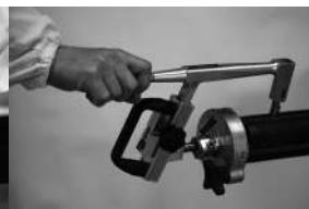
Phase 3 manual scraping
