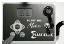
Phase 6 or setting up of parameters of manual welding
