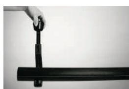
Phase 1 cutting of the pipe
