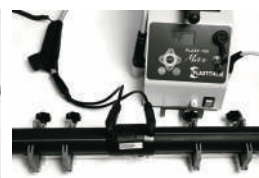
Phase 7 welding and cooling
